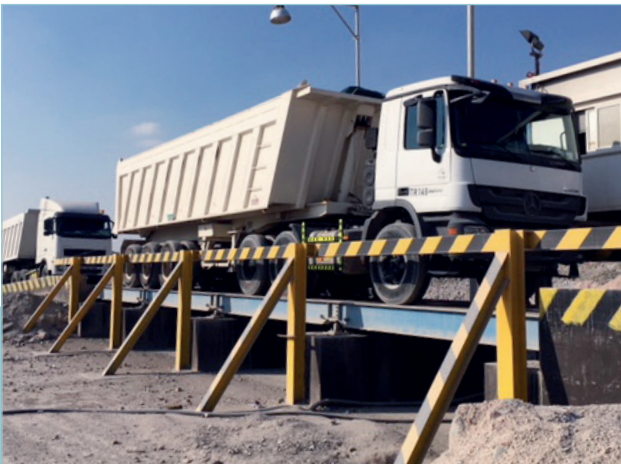
Highly durable truck scales are required for the extreme conditions at the United Arab Emirate of Fujairah
